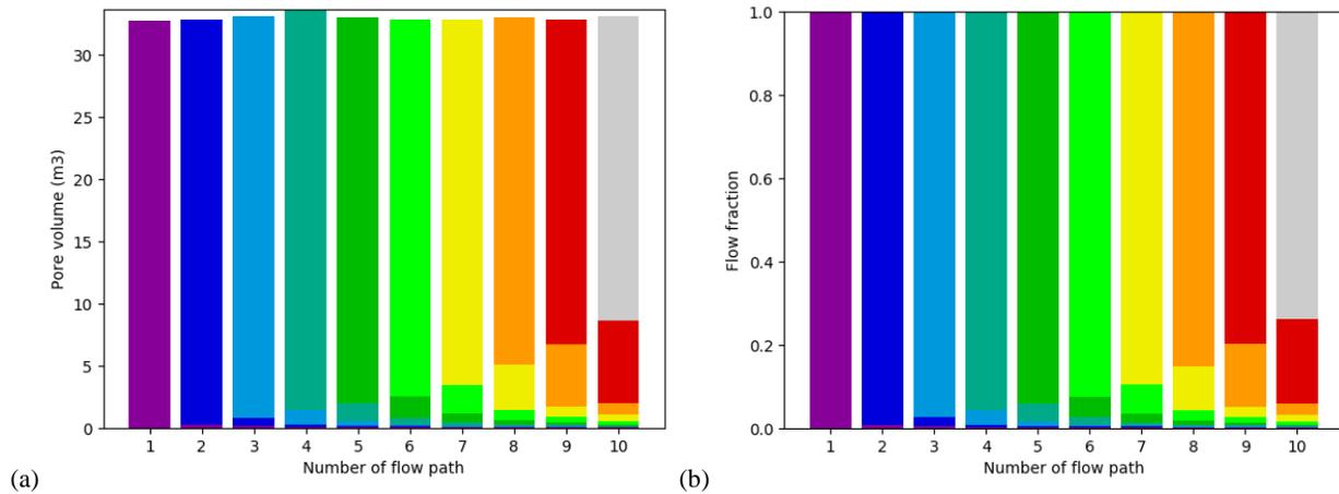
**Figure 5: Flow rate and pore volume calculated from tracer response curves. The tracer was simulated by the TOUGH2 without leakage.**
