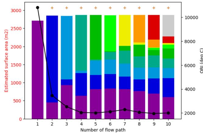
**Figure 6: Estimated results for effective heat transfer area for the simulation without leakage. The total length of bars is the estimation of the accumulated surface area. Color difference describes each surface area for each flow path. The plots of “+” describes the exact surface area of fracture zone set in the numerical simulation. The black line plots the minimum value of the objective function.**
