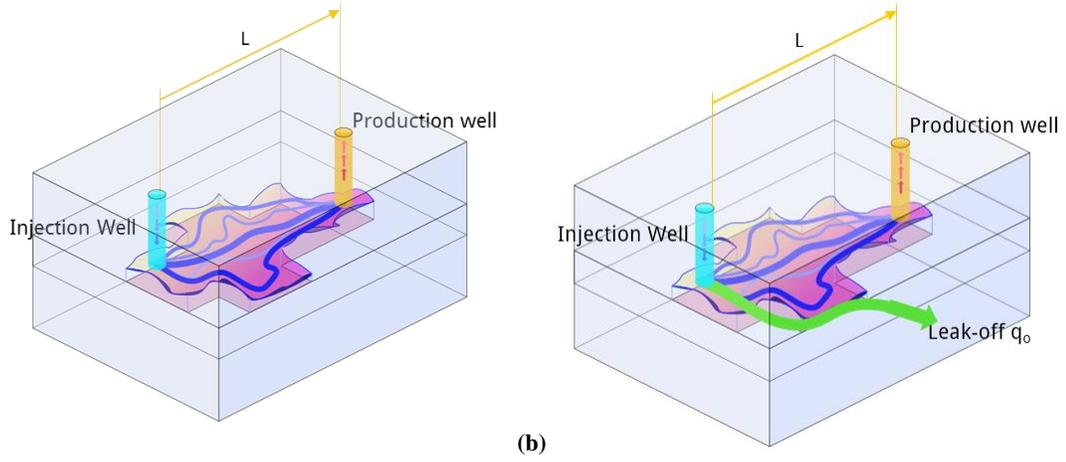
Figure 1: Schematics of the flow path model in a reservoir (a) without leakage and (b) with leakage.
