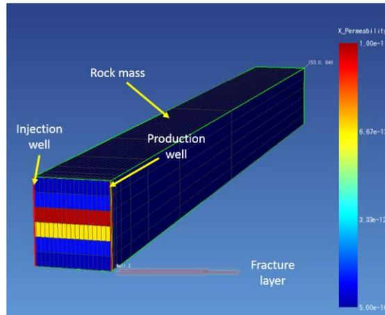
**Figure 2: Numerical model of a fracture zone with six flow paths distributed vertically.**
