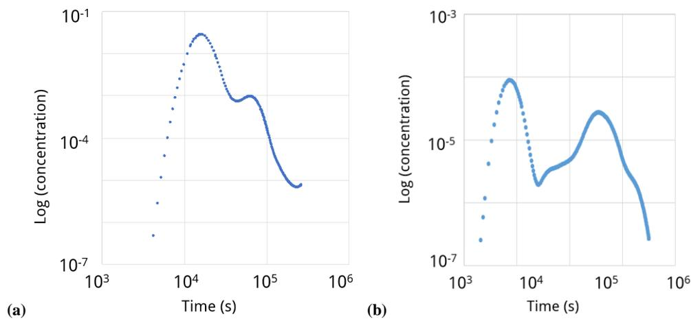
**Figure 3: Tracer response curves simulated from the TOUGH2 (a) without leakage and (b) with leakage.**
