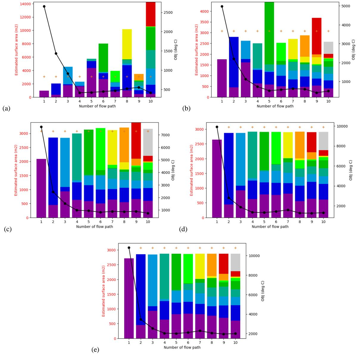
**Figure 10: Estimated results for effective heat transfer area with factor of data (a)  $\xi = 0.2$ , (b)  $\xi = 0.4$ , (c)  $\xi = 0.6$ , (d)  $\xi = 0.8$  and (e)  $\xi = 1.0$ . The total length of bars is the estimation of the accumulated surface area. Color difference describes each surface area for each flow path. The plots of “+” describes the exact surface area of fracture zone set in the numerical simulation. The black line plots the minimum value of the objective function.**
