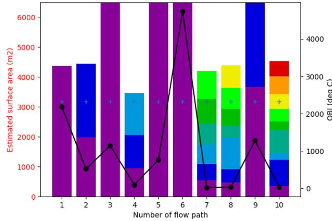
**Figure 8: Estimated results for effective heat transfer area for the simulation with leakage. The total length of bars is the estimation of the accumulated surface area. Color difference describes each surface area for each flow path. The plots of “+” describes the exact surface area of fracture zone set in the numerical simulation. The black line plots the minimum value of the objective function.**
