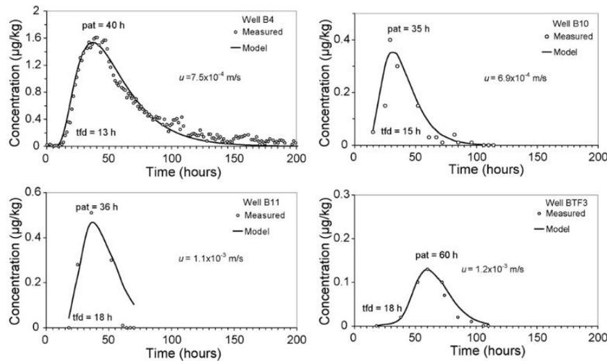
Figure 13: Tracer response curve injection at well B9 (Aksoy et al., 2008)
